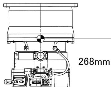
**Fig. 5-3 Center of gravity of the pump**
