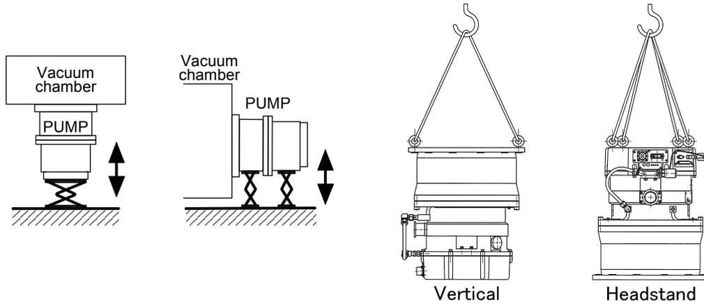
**Fig. 5-2 Lifting Method**
