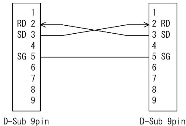
**Fig. 6-5 Example of RS-232C cable wiring connections**
