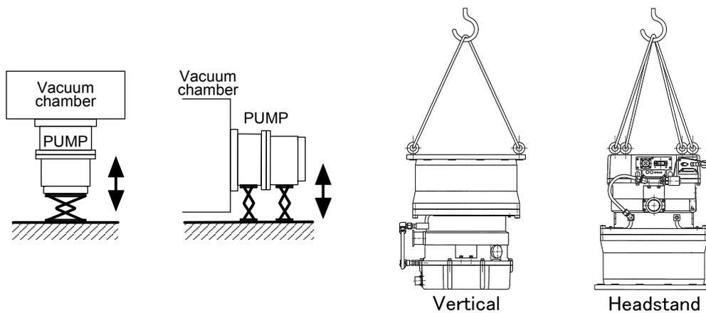
**Fig. 8-1 Way to remove the pump**
