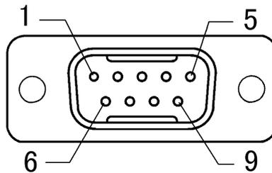
**Fig. 6-7 Serial Connector Pin Configuration**
