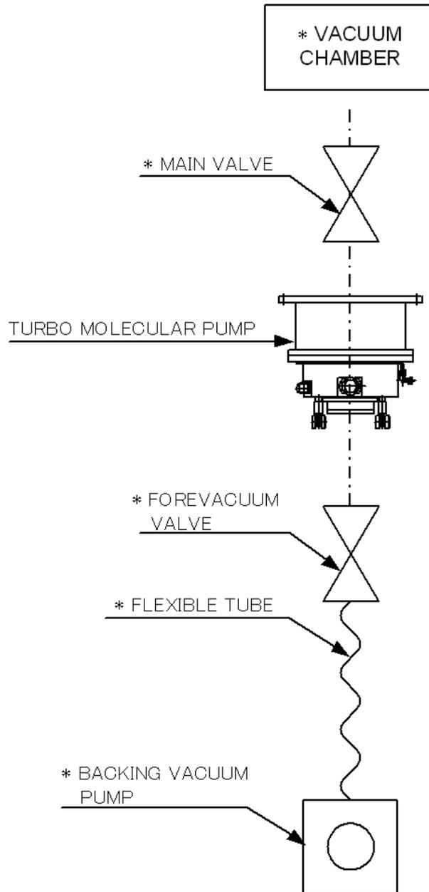
\* marks are not attached to this turbo molecular pump set.
