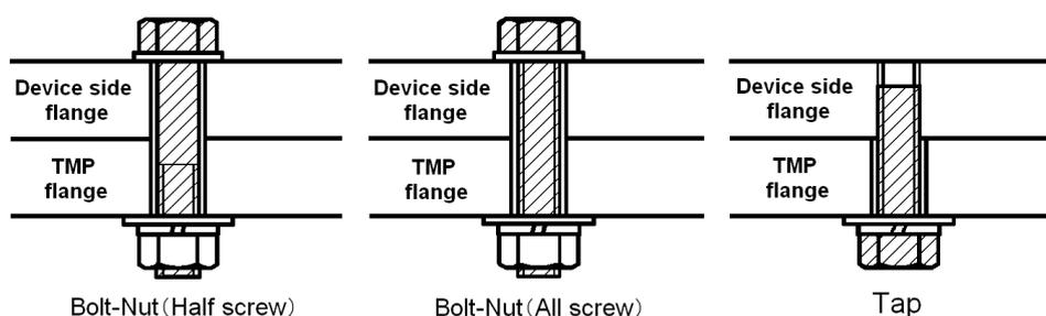
**Fig. 5-5 How to use of the bolt**
