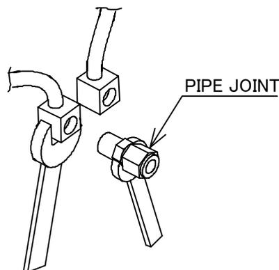
**Fig. 5-12 Water Coolant Tubing Connections**
