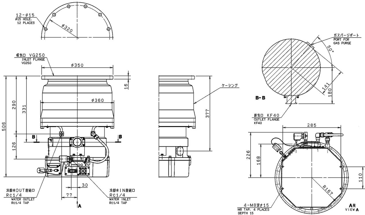
**Fig. 1-2 TMP-V2804LM/LMC (F) (VG250) Outside drawing**
