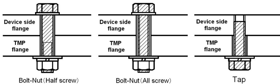
**Fig. 5-8 How to use of the bolt**
