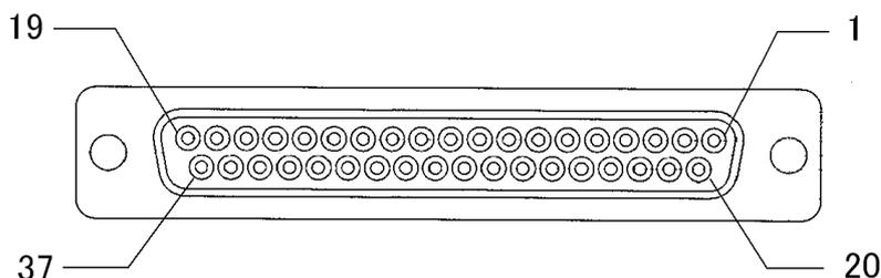
**Fig. 6-4 Arrangement of Remote-Control Connector Pins**
