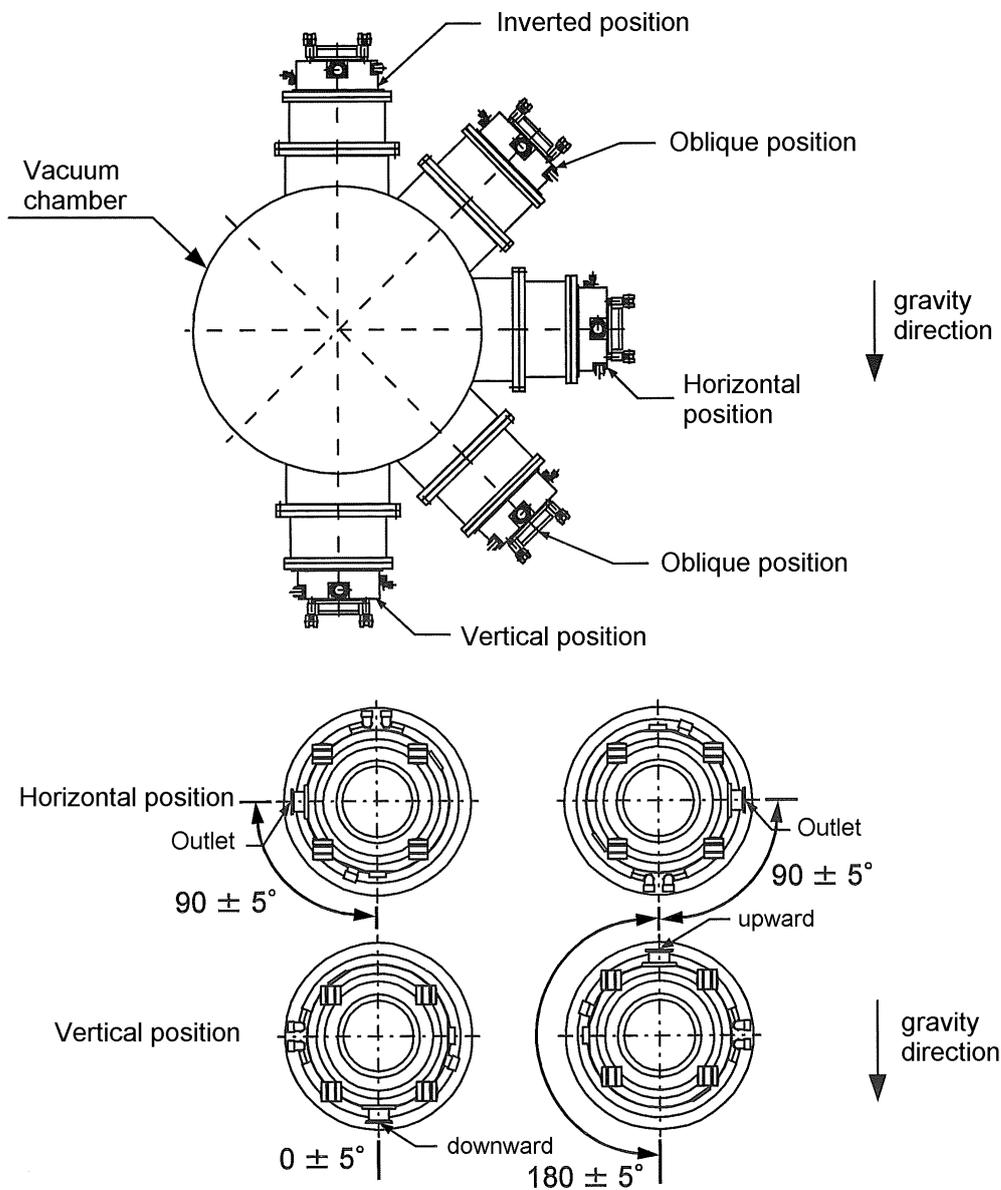
**Fig. 5-1 Mounting Direction of the Turbo Molecular Pump**
