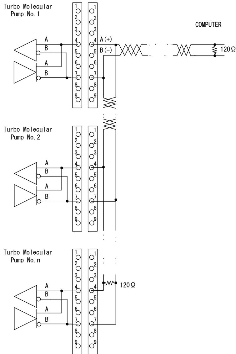
**Fig. 6-6 Example of RS-485 cable wiring connections**
