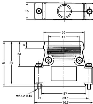
**Fig. 6-2 Remote-Control Connector**
