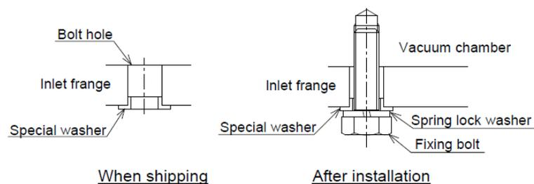
**Fig. 5-9 Example of the fixing method using the special washer**
