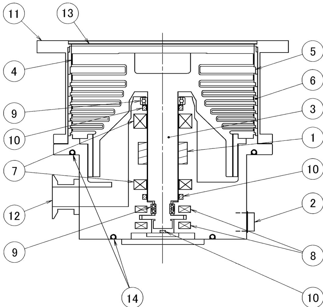
**Fig. 3-1 Pump Sectional Drawing**
