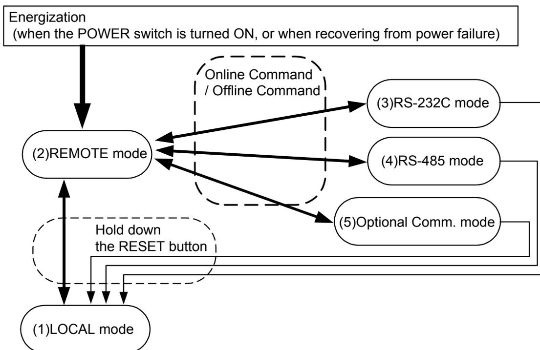
**Fig. 6-1 Operation Mode Transition Diagram**
